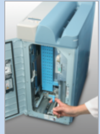
Optical unit sweeper enables self-maintenance for pristine image quality and longer product lifetime
