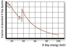
High absorption efficiency, with typical sudden increase at the Br, Sr, I and Ba K-edges of 13, 16, 33 and 37 keV
