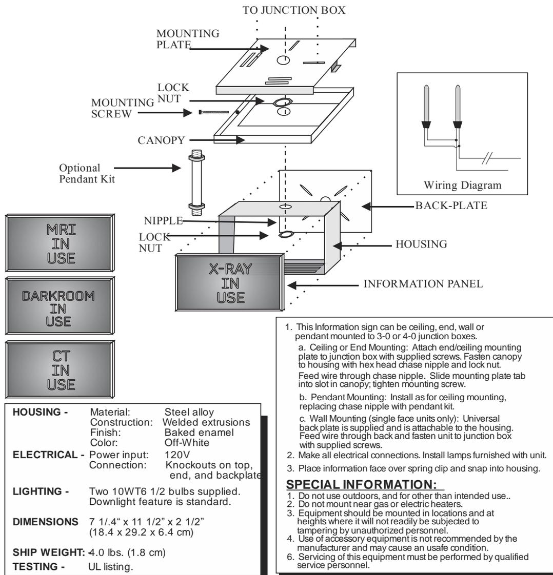
Note: LED models use two 1-Watt LED lamps – 120VAC 60Hz with 26 LED lights.
