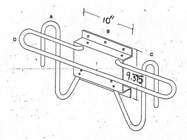
Glove-Rack Kit Add storage for 4 pairs of gloves to a Deca-Rack or 2 pairs to a Penta-Rack. Posts screw into pre-drilled holes on racks manufactured since 10/04.
