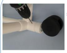
DRILL THROUGH CASTER SOCKETS USING 1/8 DRILL BIT AND PILOT HOLES AS REFERENCE.
