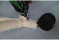
SECURE USING 1/2" RETAINING SCREWS AND PILOT HOLES AS REFERENCE.
