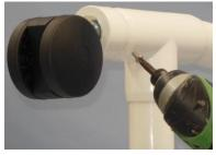
SECURE CASTERS USING 1/2" RETAINING SCREWS.
