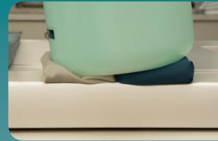
*A traditional pad (left) demonstrating bottoming out and viscoelastic material (right) showing that weight is redistributed without bottoming out*
